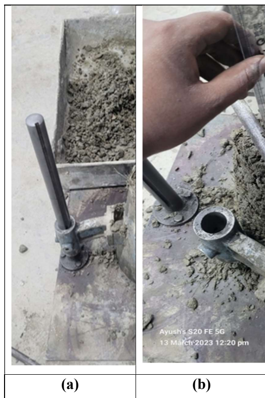
Figure 5 a) Slump test b) Measurement of slump value
