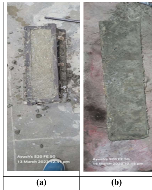
Figure 2 a) Moulding of Beam b) Concrete beam
