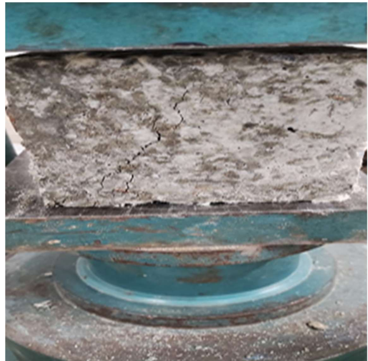
Figure 5 Cube specimen after fail
