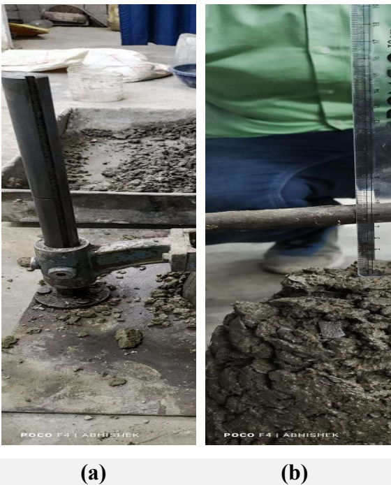
Figure 4 Slump cone test performed and reading of slump value measured
