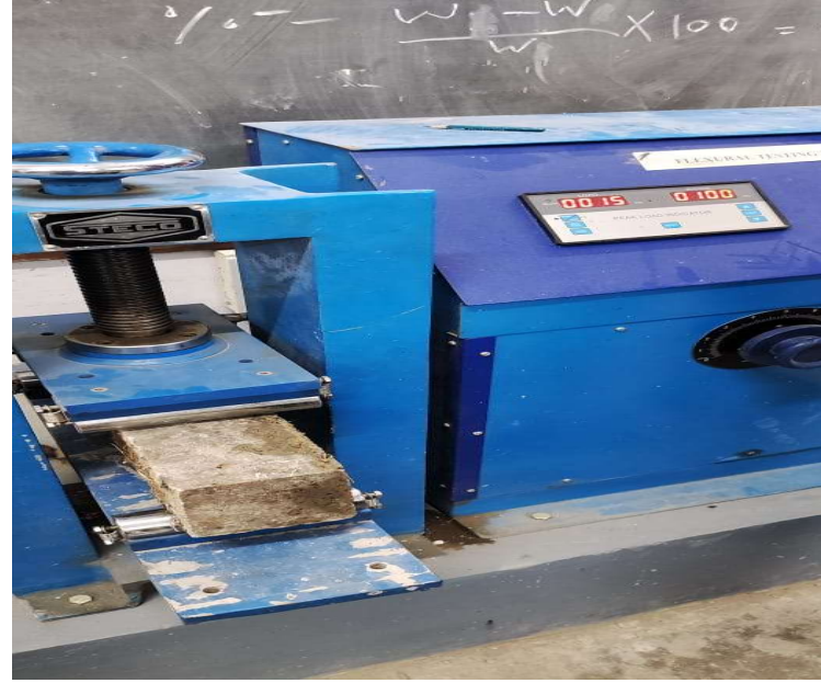
Figure 6 Load applied on beam in two-point loading arrangement
