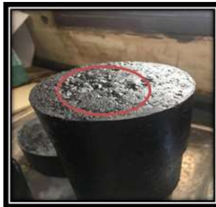
Figure(8): Raveling in MA specimen's surface.
